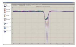
Discharge process displayed through BACS $^{\otimes}$  Viewer software shows the voltage drop of several batteries during a discharge, unnoticed by the UPS. In a later stage, these accumulators would cause the complete system to collapse! BACS $^{\otimes}$  corrects this problem and attempts to fully recharge this specific battery.
