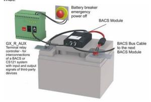
The GX\_R\_AUX module provides 4 relay contacts and 4 digital inputs. It controls up to 4 breakers. The digital inputs read the battery breaker status and display it in the BACS<sup>®</sup> web interface. Other alarm devices (for example, audio alarms) may be connected to the outputs or digital inputs of the GX\_R\_AUX.
