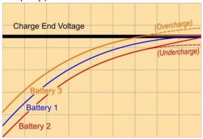
The charging of accumulators according to BACS® patented equalization process. The charging of Battery 3 is capped to prevent overcharging and gassing. Supply of charging energy to Battery 2 is continued and boosted until the target charging voltage is obtained. Battery 1 performs ideally and is not regulated.
